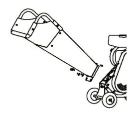
Step 5. – Connect the emergency cable. Fix the switch box by tightening the two bolts (A), and then connect the cable plug.
